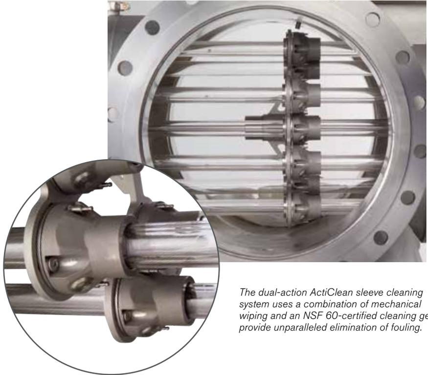
*The dual-action ActiClean sleeve cleaning system uses a combination of mechanical wiping and an NSF 60-certified cleaning gel to provide unparalleled elimination of fouling.*
